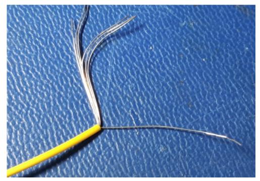
5. Solder a piece of this very thin wire across the cut groove.
