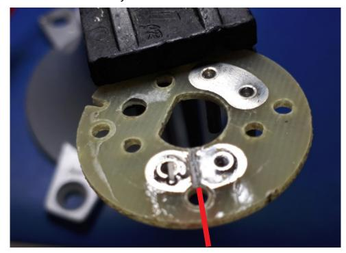
4. Separate one strand of a multi-strand wire. This will be the 5 amp fuse. Mine measures 0.006" (0.13mm).
