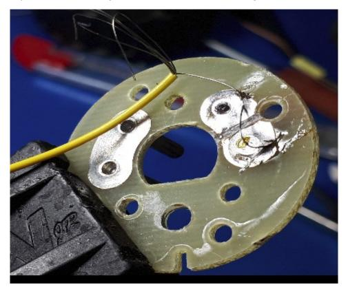
6. Drill a hole through the circuit board and the cap top. Insert a  $\#4-40 \times 3/4$ " (M3 x 20) machine screw.
